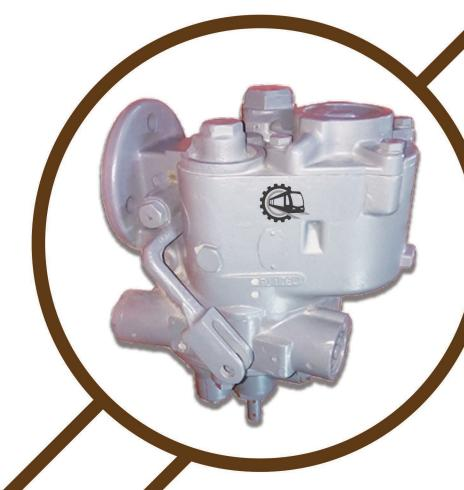
The C3W2 distributor is basically a C3W distributor with the "Empty-Load" function added, providing two ranges of brake cylinder pressure.
